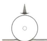
Dynamic or vibration rollers must have the vibration stopped when stationary as they would tend to sink into the surface leaving an indentation and possibly 'bow waves' on both sides on the roller.
