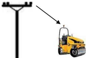
The distance you must be away from the powerlines will be determined by the voltage of the electrical lines. This can be determined by its support, if it's on wooden posts or metal pylons. This is important because certain weather conditions electric can arc (jump).
