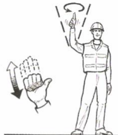
Inch load Slowly raise load or attachment Clench and unclench fingers to signal 'inch the load'
